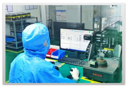
"Customers like our product for two reasons; the first one is that SENIS Mappers can measure all three components of magnetic field with unprecedented accuracy and repeatability very close to the magnet surface and in small gaps. The second reason is that our mapper software is very user-friendly and offers different types of analysis, with different types of data visualization." - SENIS AG
