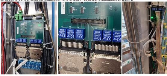
SENIS CS series current sensors offer low current sensing with high voltage isolation capability. The SENIS CS sensor incorporates the high sensitivity Hall IC and a multi-turn coil to further increase sensitivity.
