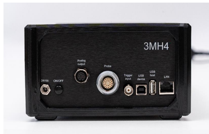
Figure 1: 3-channel digital teslameter 3MH4: front panel (left); rear panel (right)
