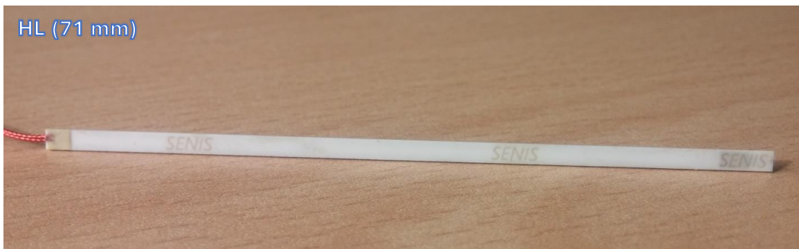
Figure 1: Photos of the 3-axis Hall probes type HS (length 8 mm), HM (length 47 mm) and HL (length 71 mm)
