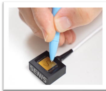
Figure 9: SENCAM with Magnetic Pen and letter "S" writing
